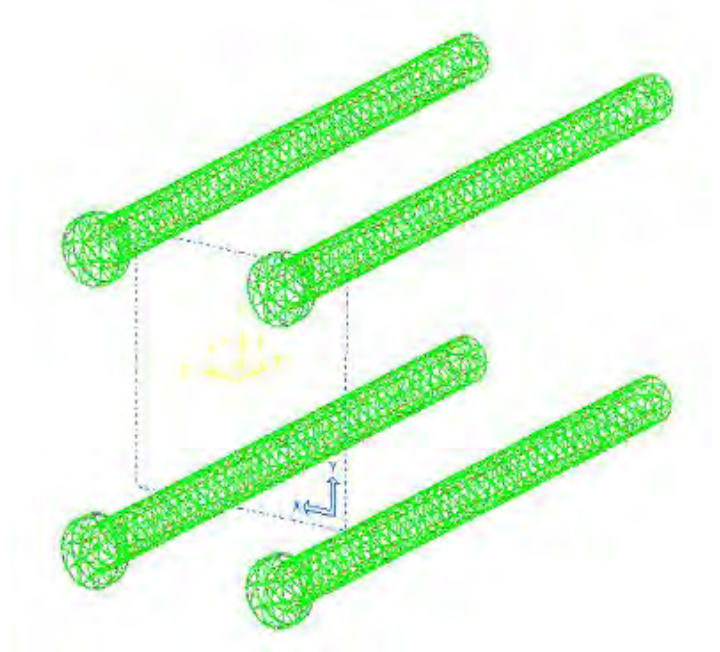
Figure 2.6: Tie Bars Mesh Model Using Solid Elements
