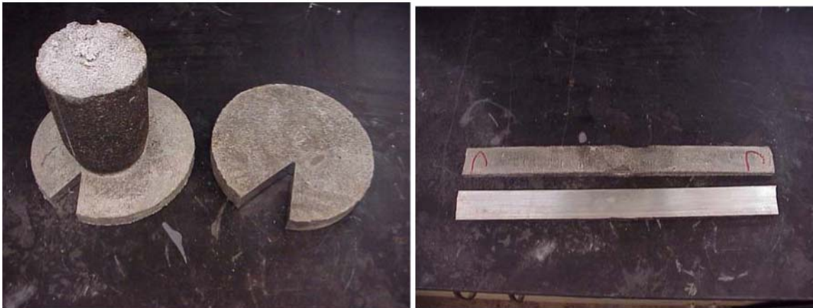
Figure 13 Sectioned small plate castings (left) and tapered bar castings (right) 5.3 15 Inch Bar Castings and MAGMA Simulation
