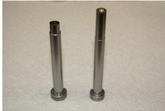
Figure 35 Example of die core pins coated with CrN/AlN based smart coatings
