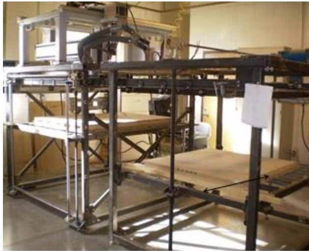
Figure 52 Additive/Subtractive Rapid Pattern Manufacturing Machine in Rapid Prototyping & Manufacturing Lab at Iowa State University
