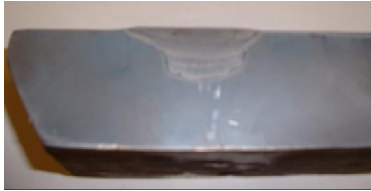
Figure 38 Picture of sample 5Q with no PWHT from alloy 8620.
