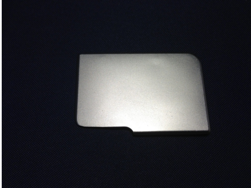
Figure 9 Surface appearance of prototype smartphone case, glass bead shot peened and surface treated to give “natural metal look”
