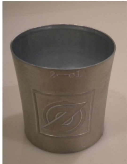
Figure 7 Business card case, thickness 0.3mm cast by Ka Shui, Shenzhen, China (l) and Cast “shot glass”, thickness 0.3mm cast by Havelleandischer Zinkdruckguss, Premnitz, Germany
