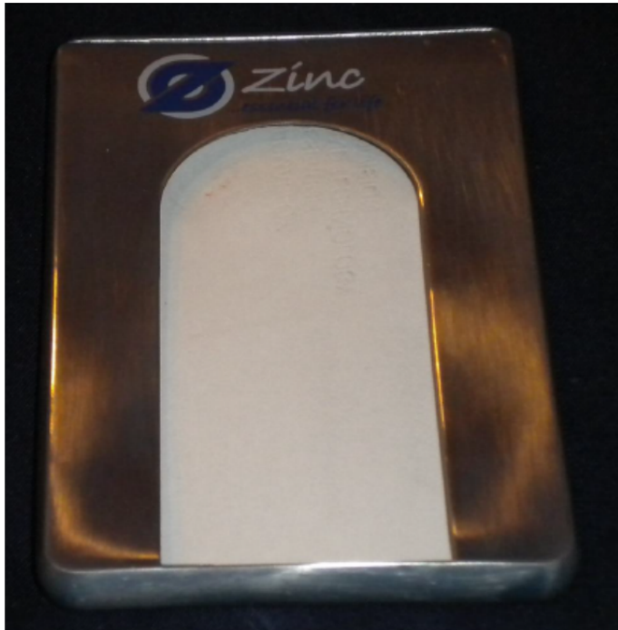
Figure 7 Business card case, thickness 0.3mm cast by Ka Shui, Shenzhen, China (l) and Cast “shot glass”, thickness 0.3mm cast by Havelleandischer Zinkdruckguss, Premnitz, Germany
