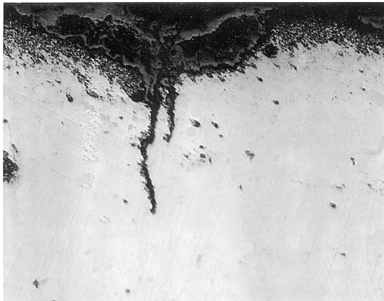
Figure 42 Crack at the Cooling Line of H13 Specimen
