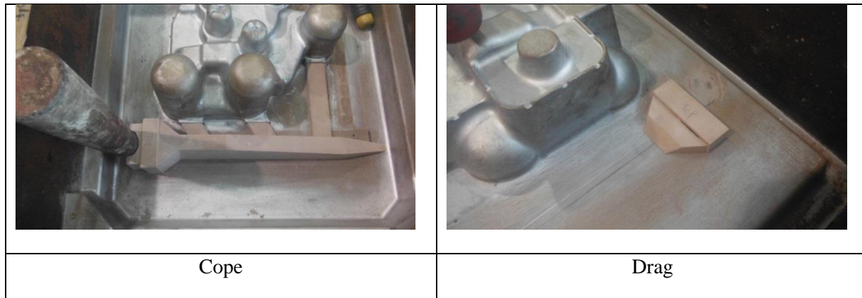
Figure 20 – Pattern pictures of pressurized gating (G3).
