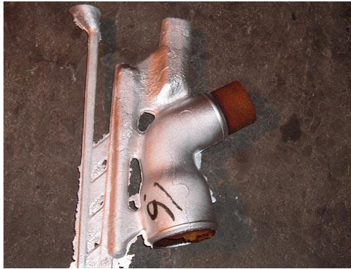
(a) Casting with gating system and core.
