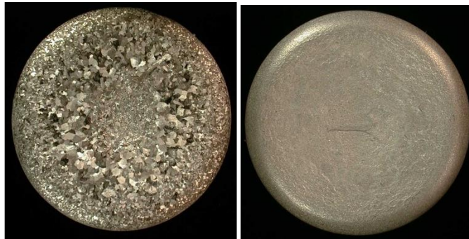
(a) Before refinement (b) After grain refinement with Ti/B
