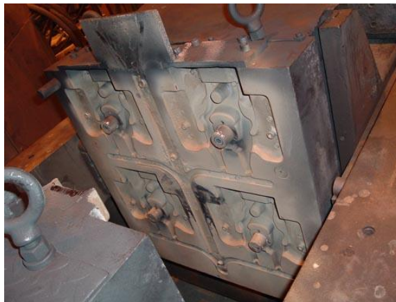
Figure 4.5.1 Mounted 4-cavity swivel mold on tilt-pour machine.
