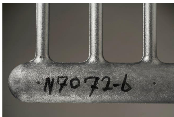
(b) N7072-6, 445°C, 0.043%Ti, no hot tear.
