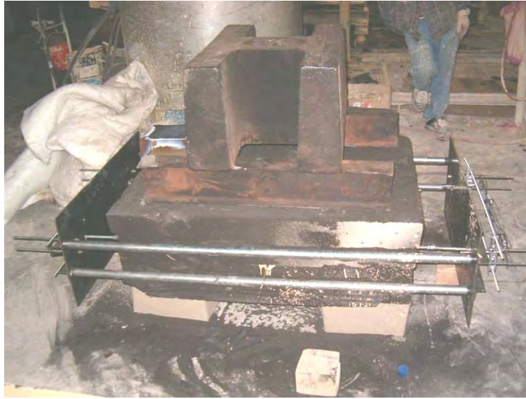
Figure 5. Flask assembled around the T-section casting mold.
