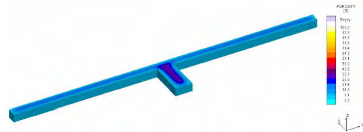
Figure 7 Porosity due to Solidification Shrinkage and Liquid Flows.
